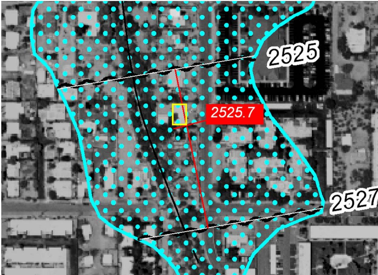
For Zone AO floodplains, obtaining a LOMC document to remove a structure or a property from the floodplain can be very difficult. The Zone AO floodplain is an approximated floodplain with average depths of flow of 1, 2, or 3 feet used instead of BFEs.
