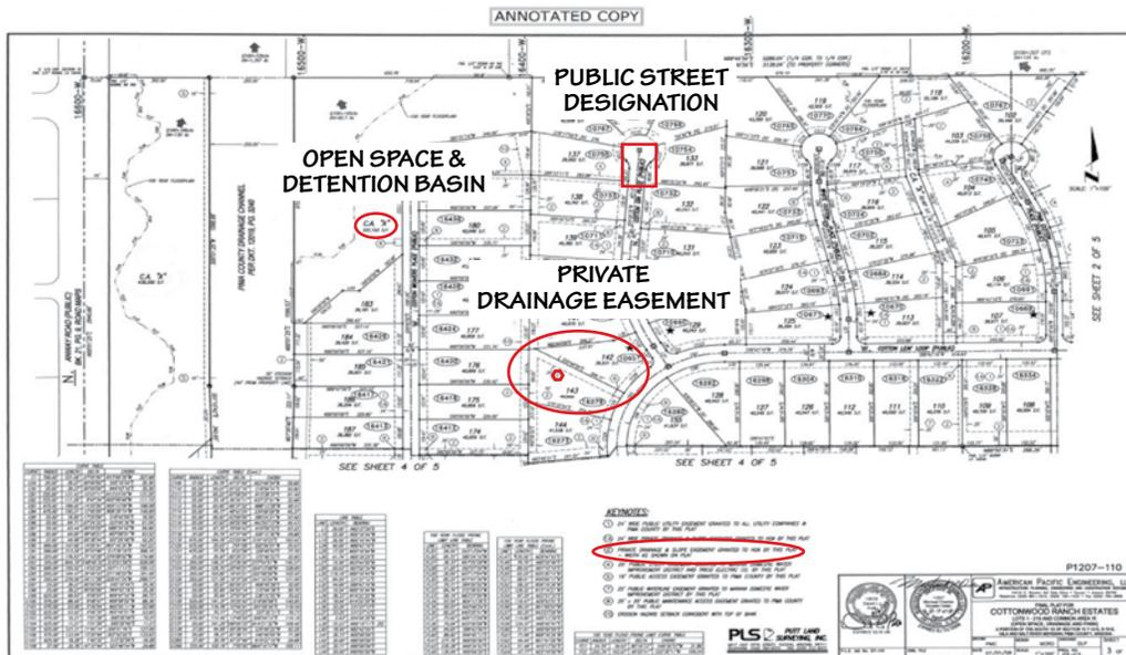
An Example Final Plat with Common Areas and Easements for Drainage
