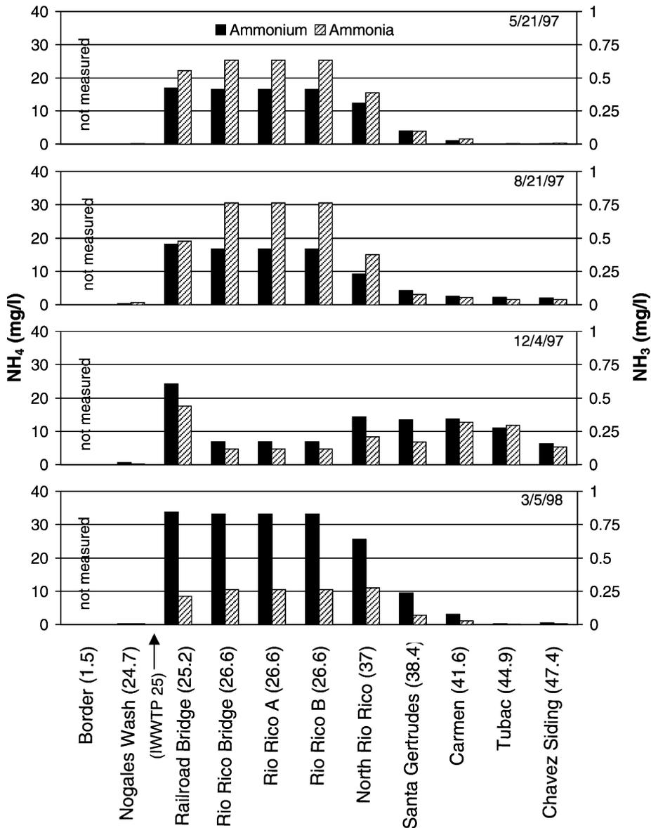
Fig. 7. Ammonium and ammonia on four dates at nine sampling sites along the upper Santa Cruz River. Numbers on x-axis refer to distance downriver from the US–Mexico border as illustrated in Fig. 2 and indicated in Table 1.
