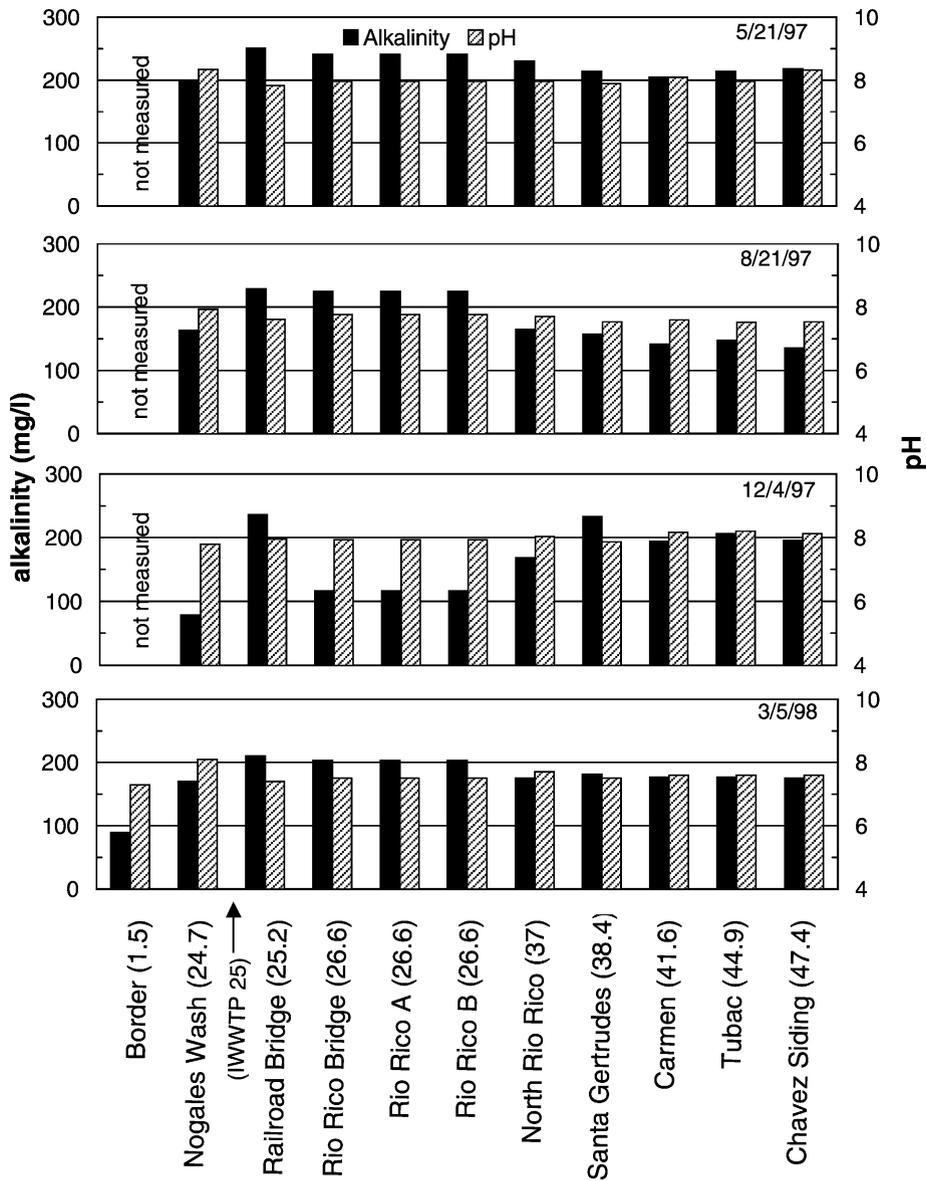
Fig. 8. Alkalinity and pH on four dates at nine sampling sites along the upper Santa Cruz River. Numbers on x-axis refer to distance downriver from the US–Mexico border as illustrated in Fig. 2 and indicated in Table 1.
