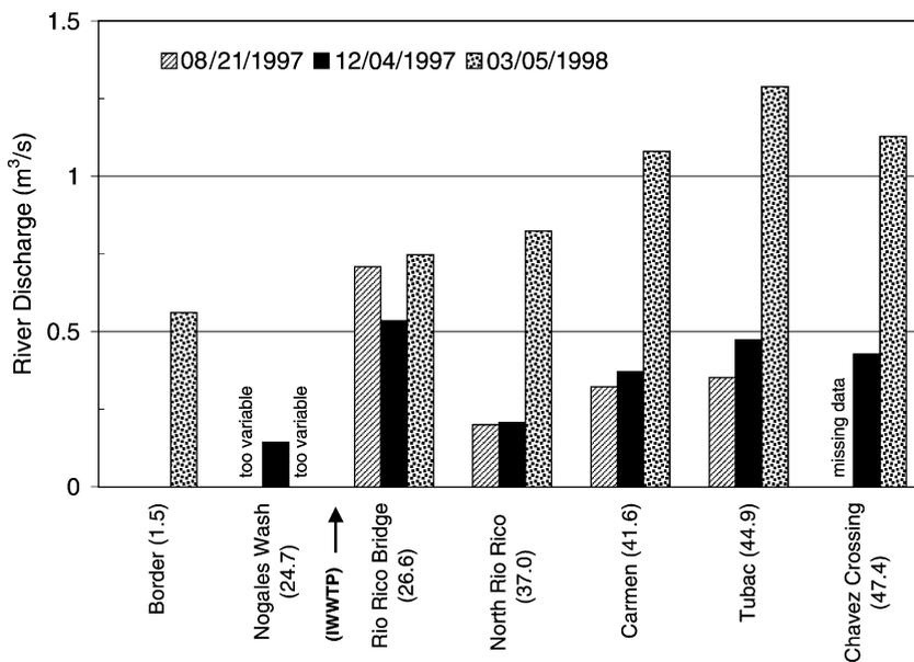
Fig. 3. River discharge measured at seven sampling sites on three dates. Numbers on x-axis refer to distance downriver from the US–Mexico border as illustrated in Fig. 2 and indicated in Table 1.
