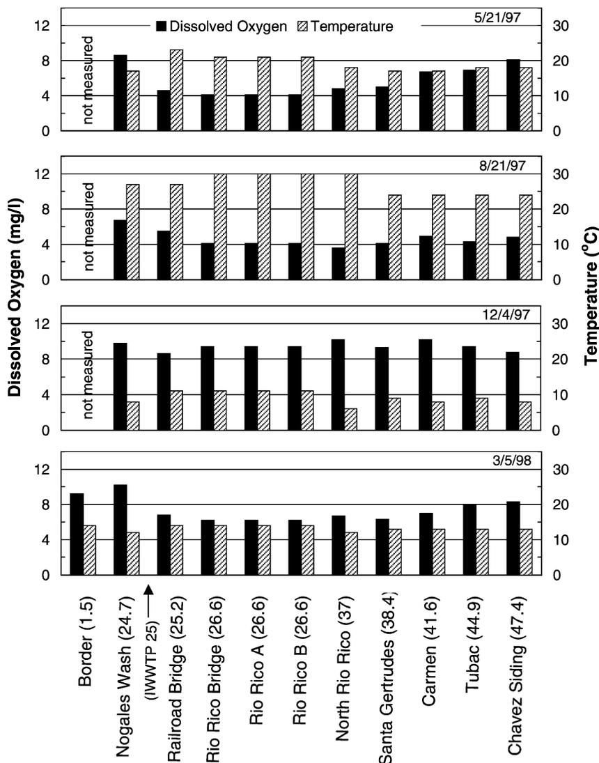
Fig. 6. Dissolved oxygen and temperature on four dates at nine sampling sites along the upper Santa Cruz River. Numbers on x-axis refer to distance downriver from the US–Mexico border as illustrated in Fig. 2 and indicated in Table 1.
